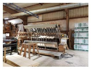
To name a few: there was a gluing machine, clamping machine, sewing machine that used glue thread for stitching veneer together, and, of course, their newest addition-the new CNC.
